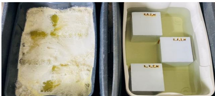
Figure 1: Test cubes immediately after placing in 20% hydrochloric acid (left side: uncoated; right side: coated). Source: own editing
