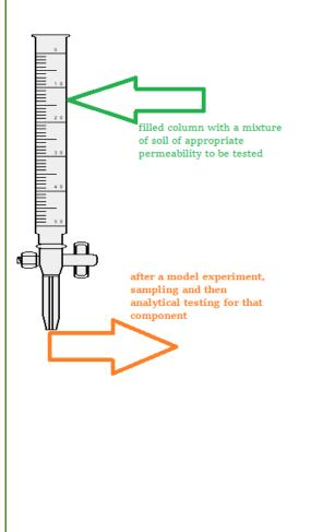
A charged model column is designed for the experiment. The column can be filled with soil samples of different permeabilities, even mixed with an artificial part (debris, concrete). The permeability of the charge is optimal if it can pass a minimum of  $1 \text{ cm}^3$  of solution per minute.
