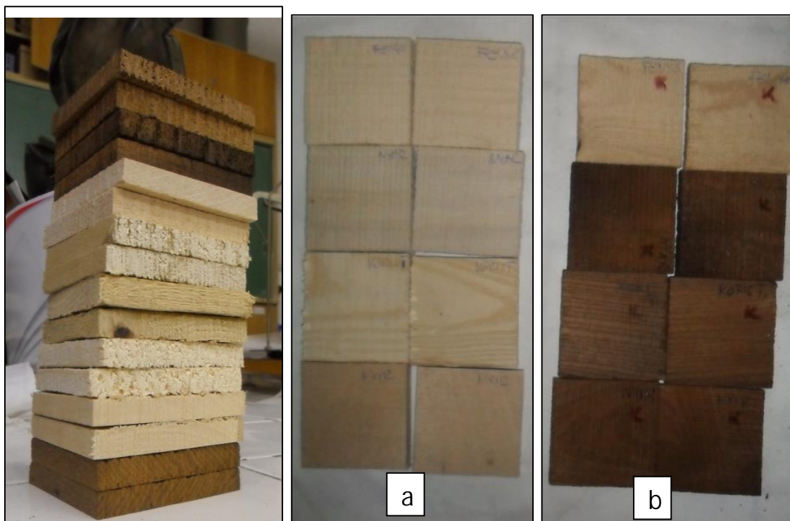
Figure 1 - Test specimens a ) untreated, b ) treated (modified). Created by the Authors.
