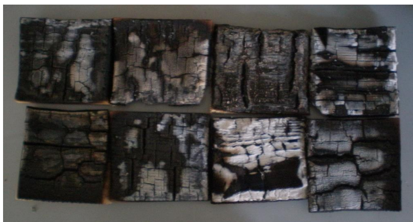
Figure 18 – ( 2 \text{ W/cm}^2 ) All of the specimens after ignition. Created by the Authors.
