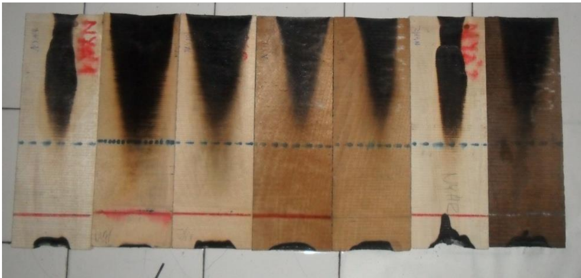
Figure 17 - Some specimens of the vertical flame propagation rate after the test. the Authors.
