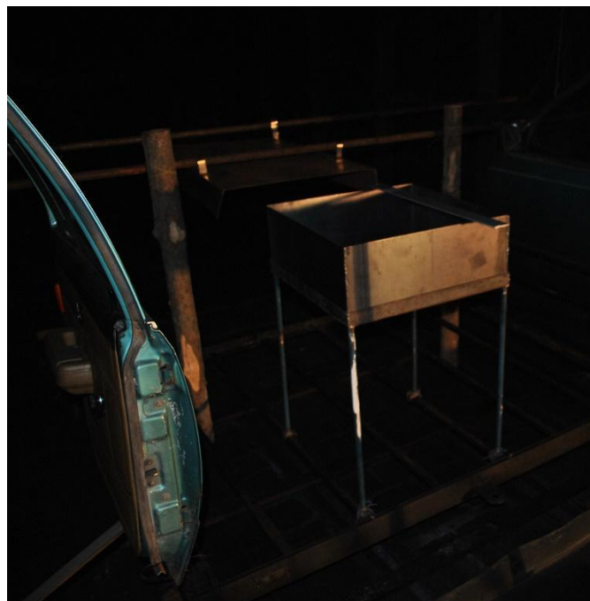
Figure 5 - Position of the door and the ignition source before the experiment
