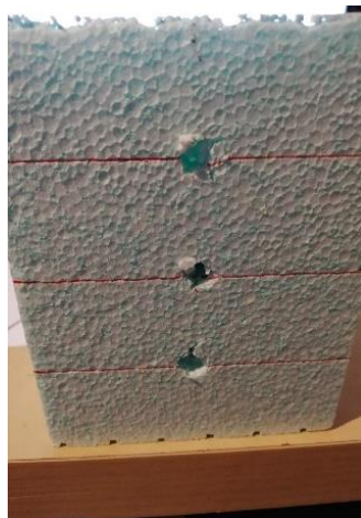
Figure 3 - Thermo elements in the specimen. Source: Authors.
