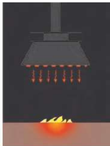
Figure 11. Energy balance on a surface. The figure shows how heat exchange occurs from the object, as well as how thermal conduction takes place through the object.
