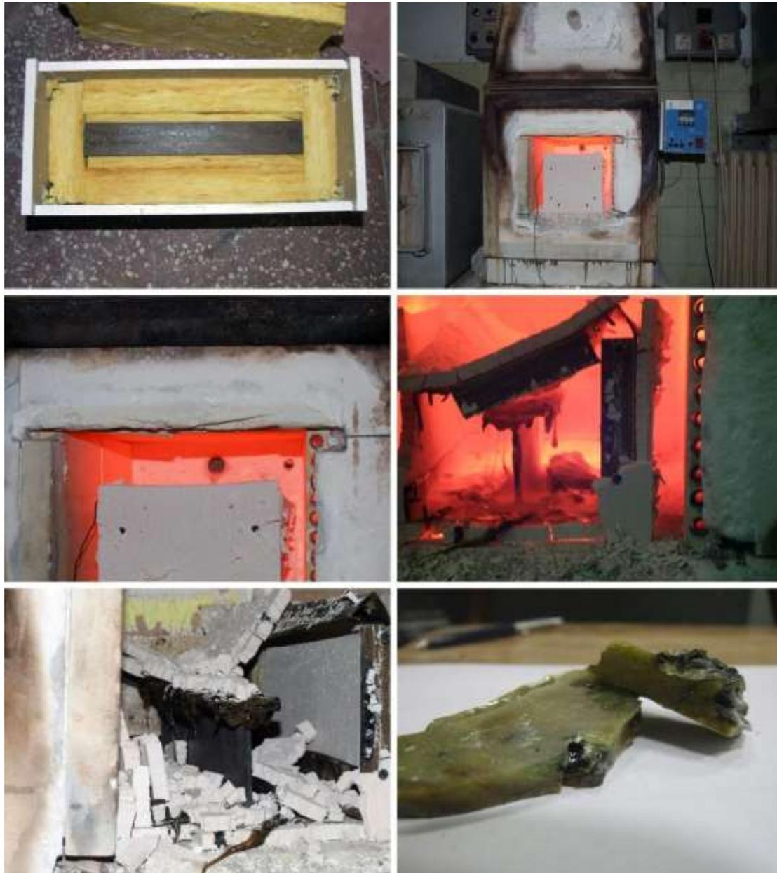
**Figure 3-** Typical failure of fiberglass insulation.
