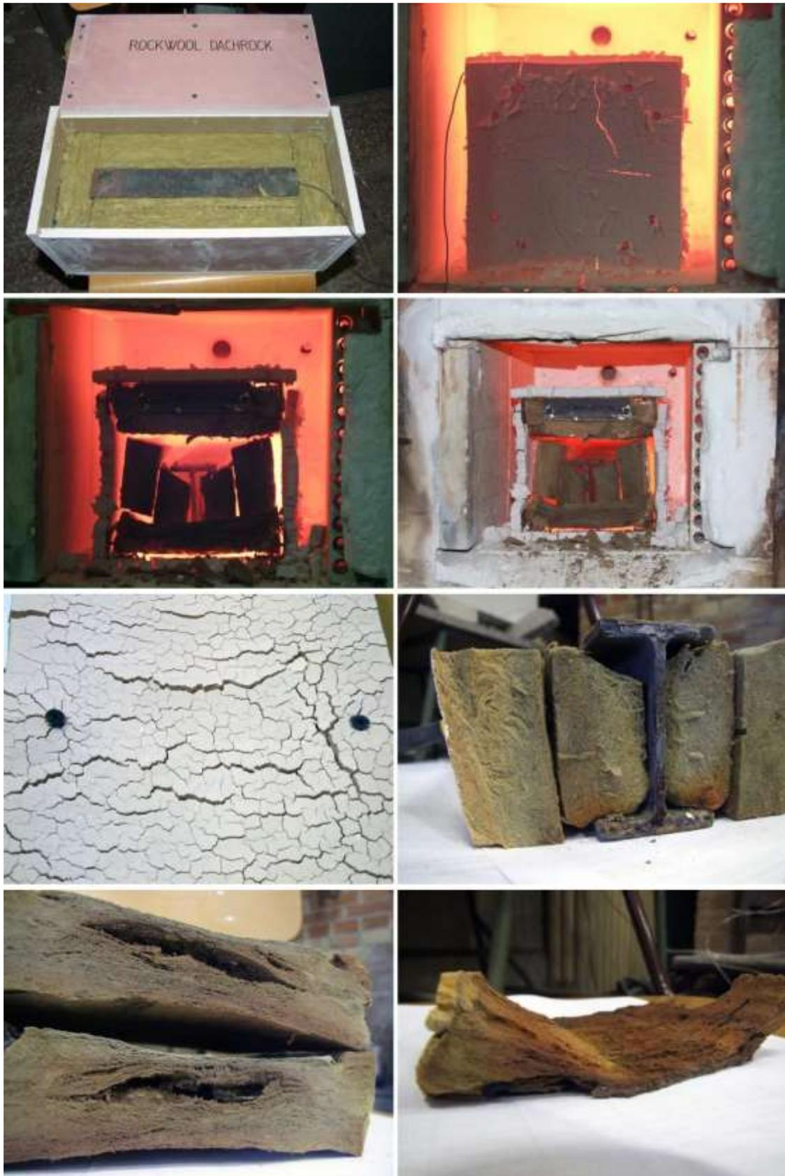
**Figure 5-** Typical failure of rock wool insulation.
