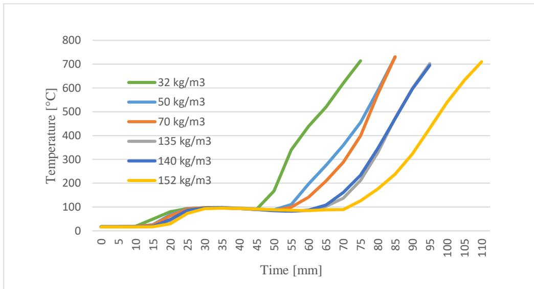
**Figure 6** - Temperature development of the steel profile in case of rock wool insulation as a function of the time
