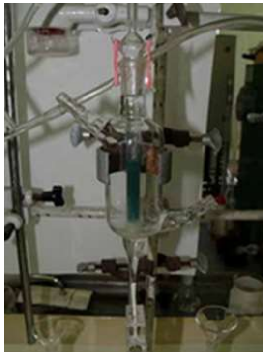
Figure 2. The laboratory ion exchange column
