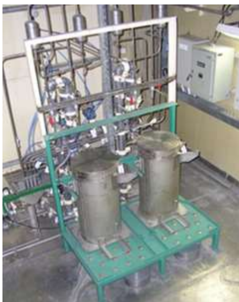
Figure 4. The 12L sorbent columns in lead shield
