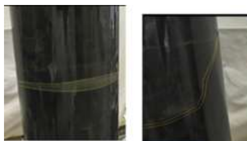
Figure 8. Channelling during high flow rate
