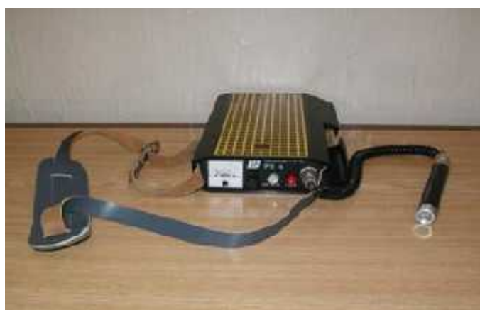
Figure 2: Detector for combustible gases and vapours PD-6
