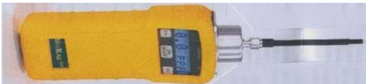
Figure 5: MiniRAE 2000 photoionization detector
