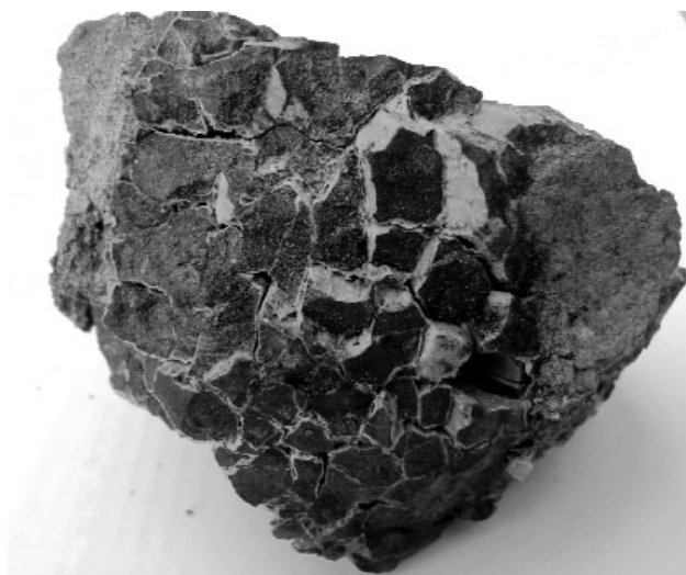
Figure 4. Phillipsite-Na crusts in the cracks of natural coke. Bátonyterenye coal mine, Hungary. Width of the picture: 8 cm
