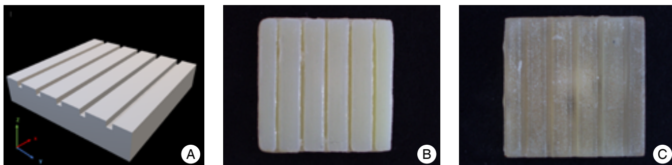
Figure 1: Three-dimensional test specimen (A), VeroGlaze Med620 stereomicroscopic image (B), Dental SG stereomicroscopic image (C)
