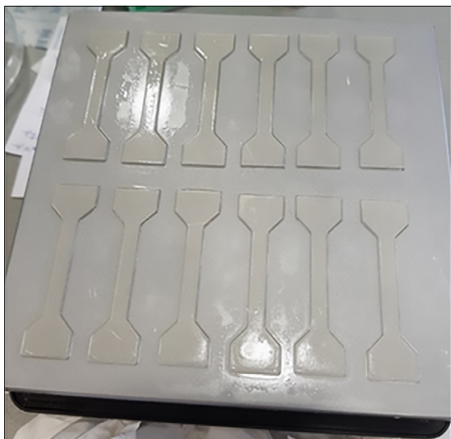
Figure 5: 3D printed specimens from experimental resin
