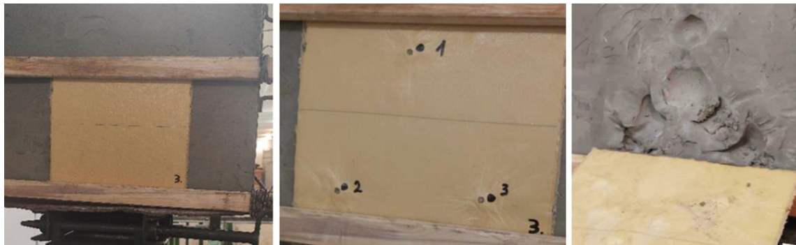
Figure 1. Ballistic testing of a self-developed composite material (Kondor et al., 2025)
