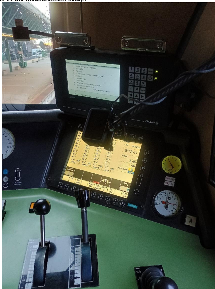
Figure 1. The measurement setup (there is the GoPro camera in front of the displays; here its display is in stand-by mode because the energy consumption is much less than with switched on display)
