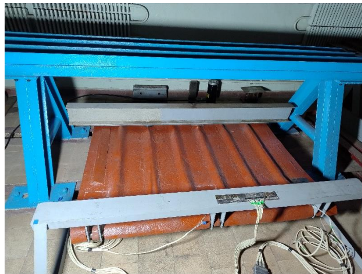
Figure 16. The placement of the hatch cover on the test stand
