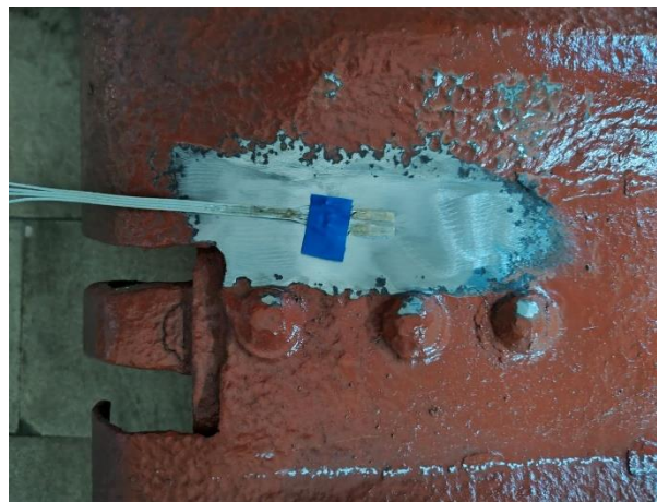
Figure 14. Placement of strain gauges on the hatch cover
