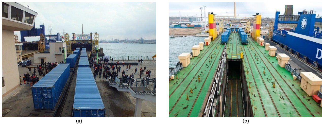
Figure 1. Transportation of flat wagons loaded with containers on railway ferries: (a) rolling of flat wagons onto the railway ferry (Makeev, 2025); (b) placing of flat wagons on the railway ferry (European Pravda, 2025).
